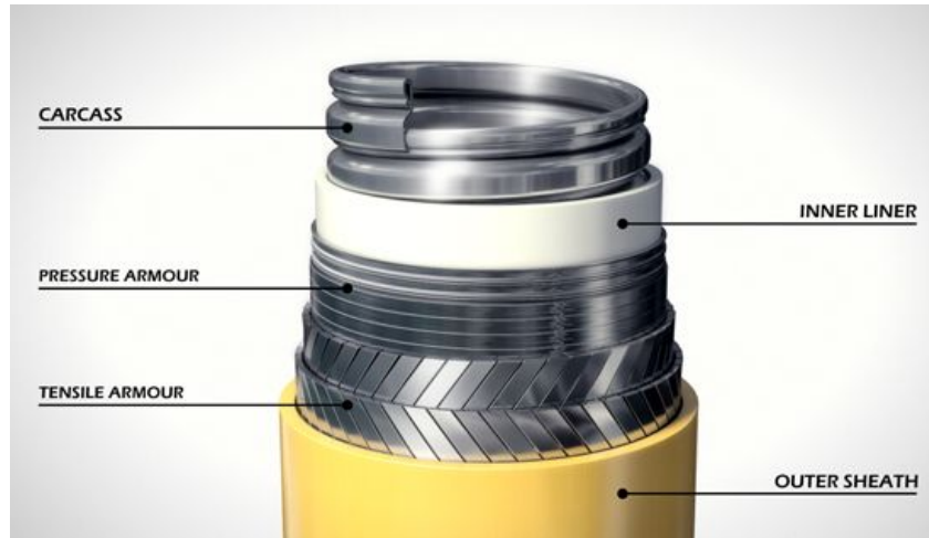
Figure 1.2.1. Flexible pipe riser construction [6]
