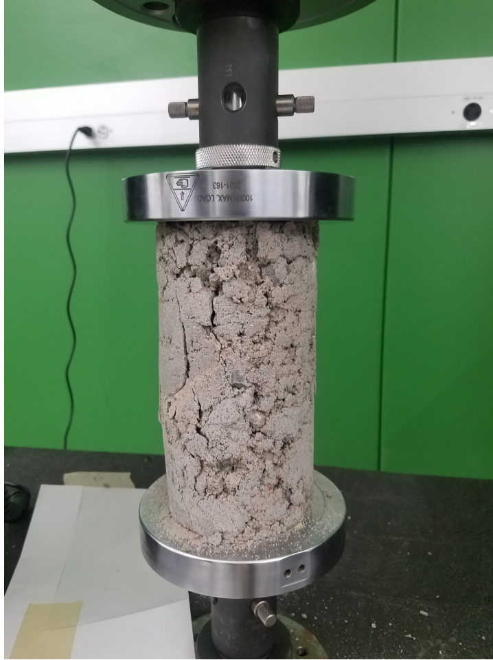
Figure 18: A Compression Sample Post Failure
