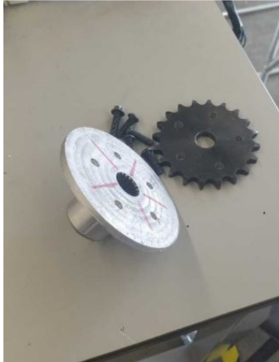
Figure 52: Custom Rear Sprocket Assembly
