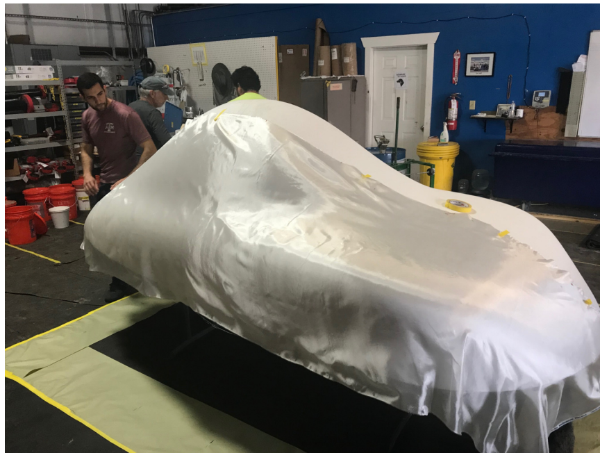
Figure 10: Top Mold Fiberglass Lay
