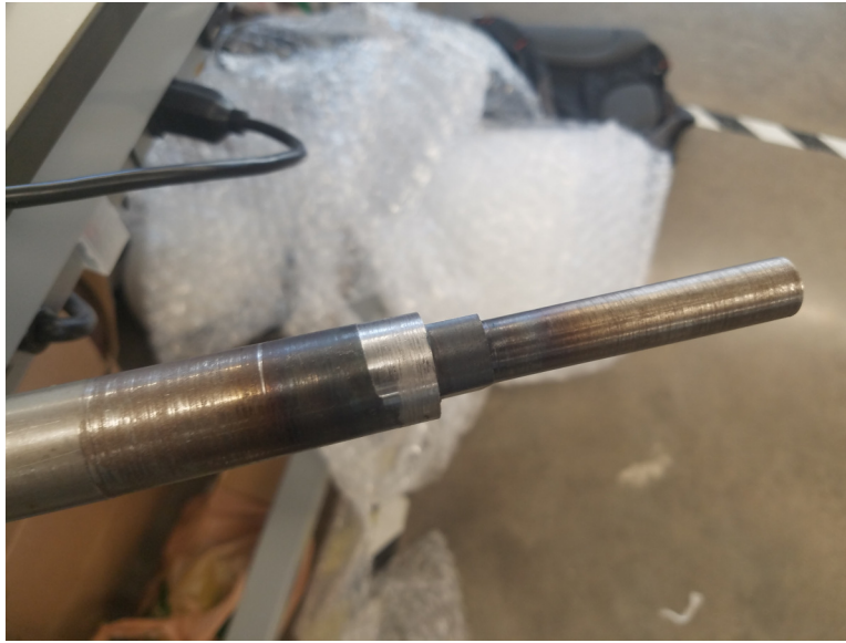
Figure 71: Axle Tip Welded and Machined
