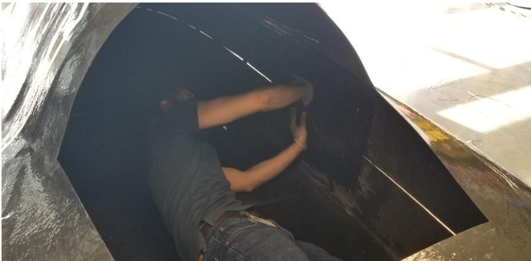
Figure 20: Door Carbon Fiber Layup
