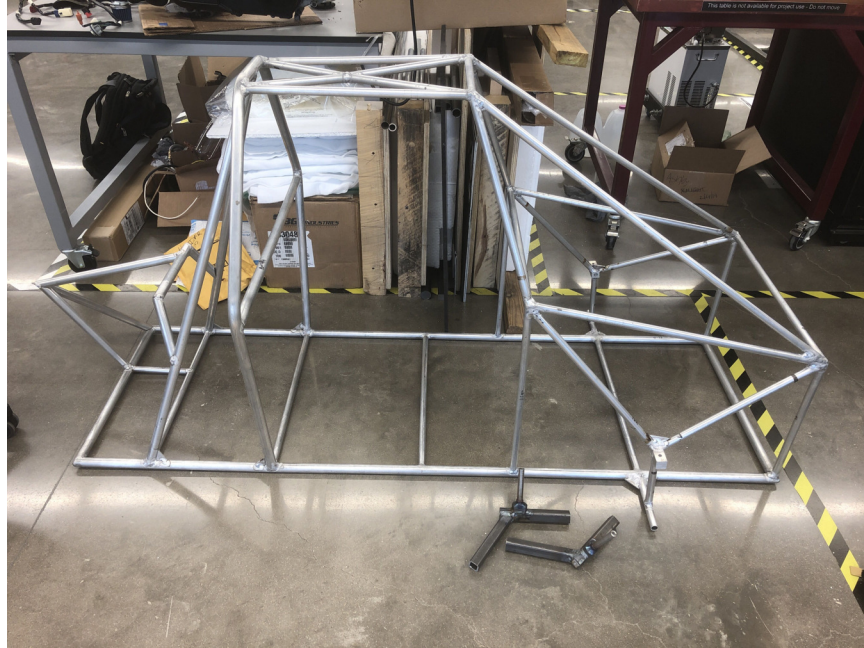
Figure 47: Frame Phases 1-10 Constructed
