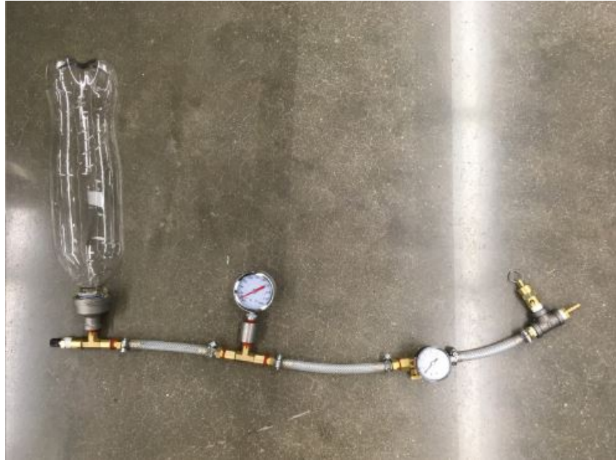
Figure 50: Fuel Delivery System according to SEM rules
