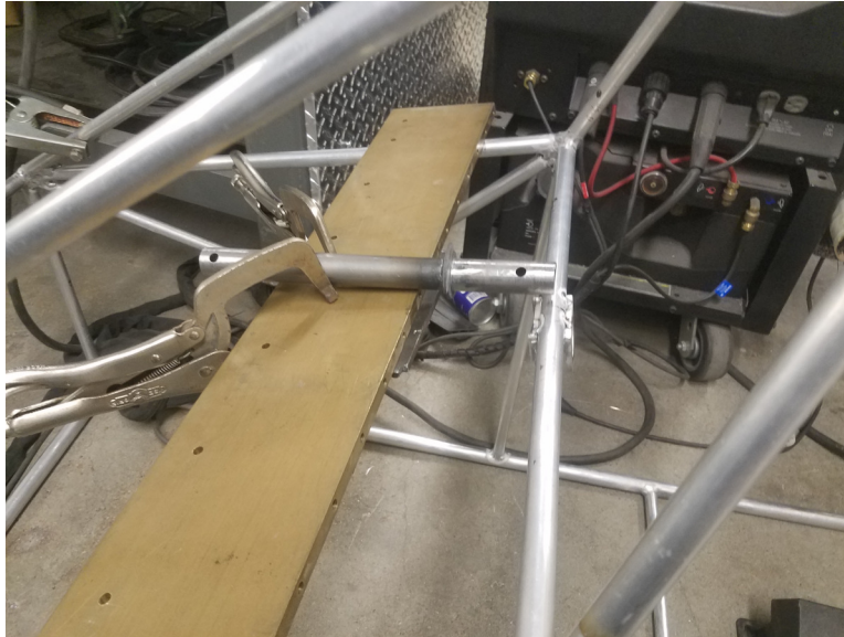
Figure 75: Welding Jig to hold Steering Hangers
