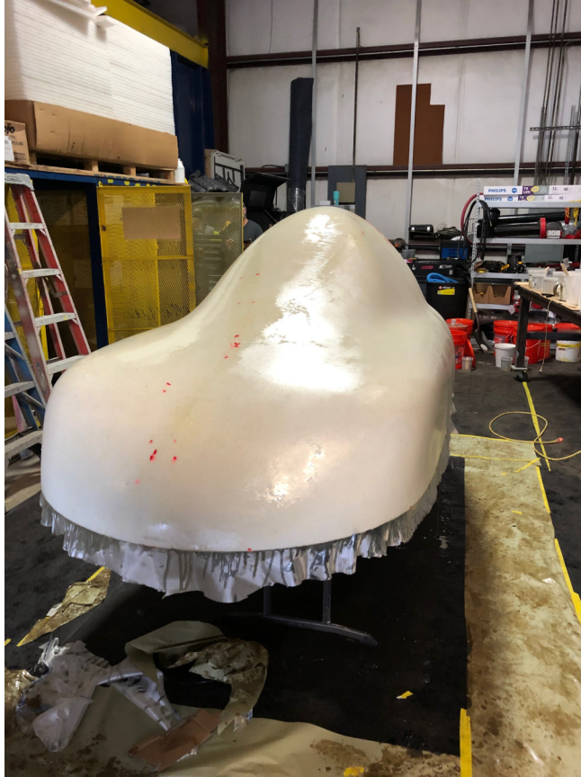
Figure 11: Top Mold First Fiberglass & Epoxy Layer
