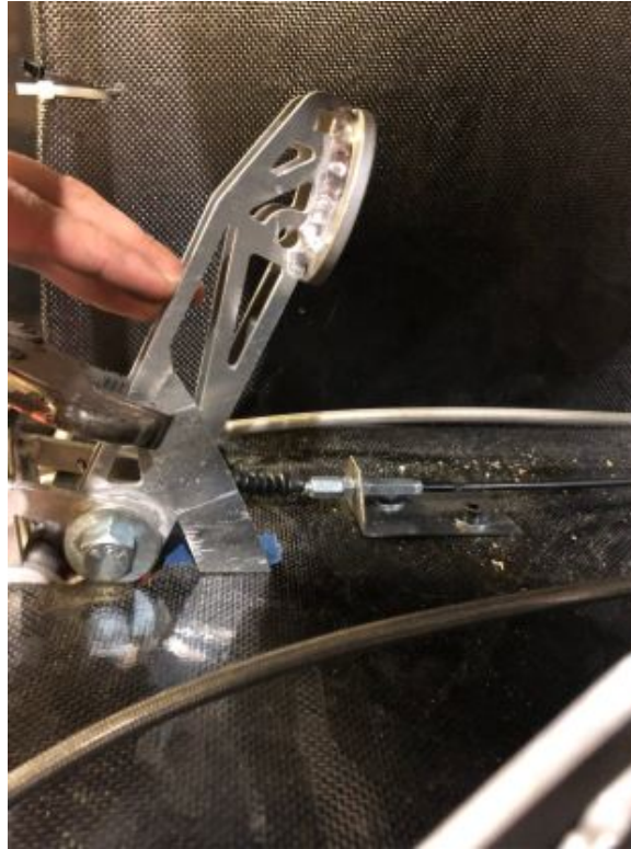
Figure 51: Accelerator Pedal and Throttle Cable
