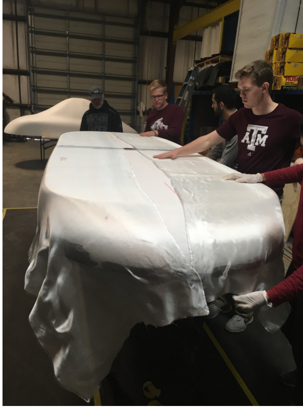
Figure 9: Bottom Mold Fiberglass Lay
