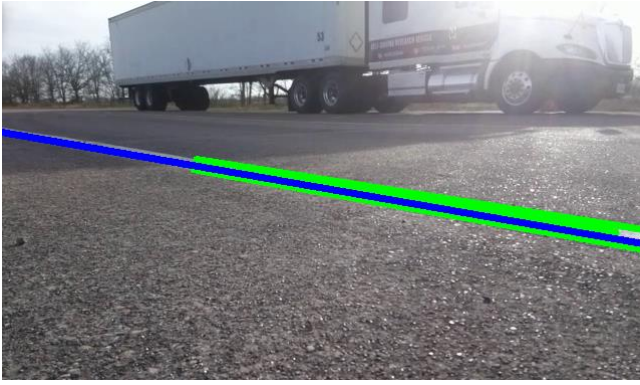
Figure 13. Results of Hough Line Transform
