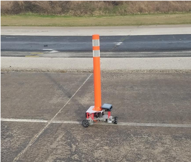
Figure 15. Cone Stopping on Line with Feedback Control
